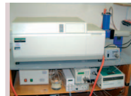
LC-CD for the acquisition of CD spectra of compounds. This is used in tandem with computer-chemical methods to elucidate the exact configuration of chiral molecules.
